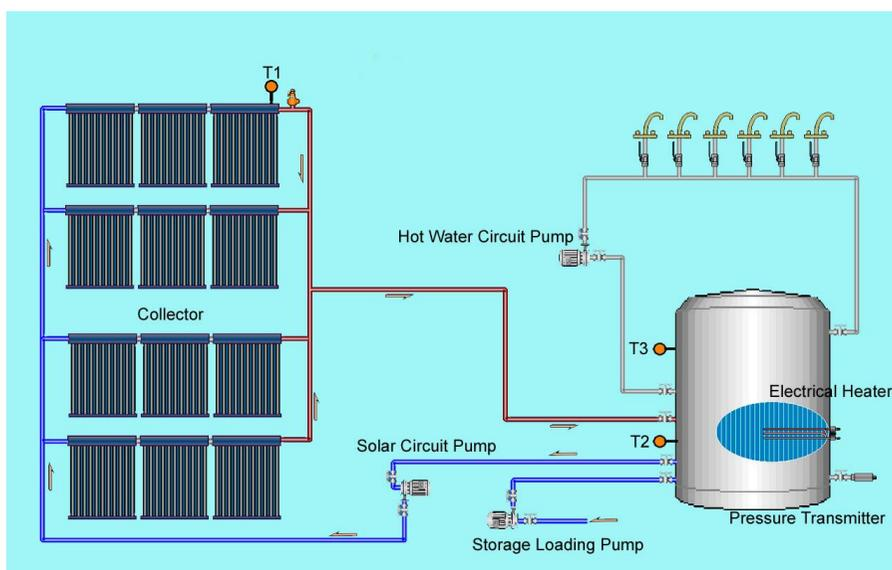
**Note:** T3 is an optional sensor, when no T3 sensor is installed in the system (no connection to input port); controller will use the signal of temperature T2 automatically to control the back-up heating or circulation.
