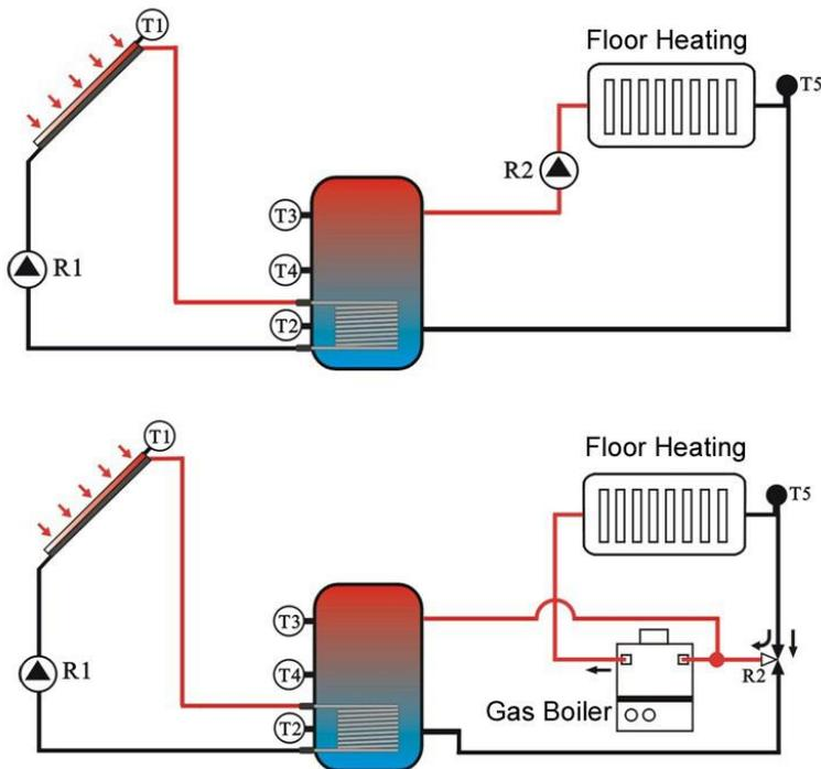
**5.5.6 AHEA Switch-on/off control of back-up heating system**
