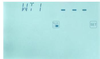
▶ Press "+/-" button to adjust the water loading temperature, adjustable range (10°C ~95°C), after activate the function, factory set is 50°C
