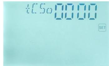
▶ Press button “+”, “tC 5F 00:00” displays on screen, the switch-off time for the fifth schedule of DHW pump function can be set.
