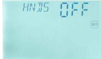
▶ Press “+” button, “HND6 off” displays on the screen, R6 output manually set
