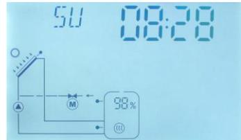
After setting and wait for 6 seconds to save the parameter automatically. Current time and week are displayed on the controller.
