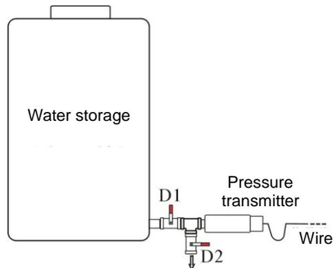
**Mounting the pressure water level transmitter**
