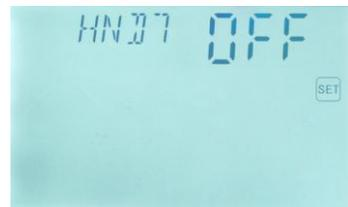
**Note:** when manual mode is activated,
